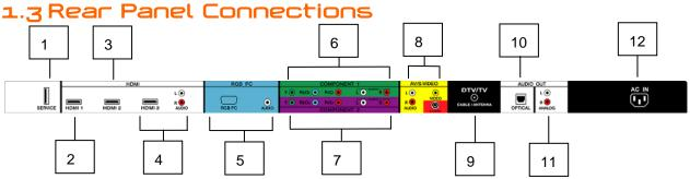
1. SERVICE – This custom communication port is for factory service only. Use of this input for any purpose other than factory authorized service will void the manufacturer's warranty of this equipment.
